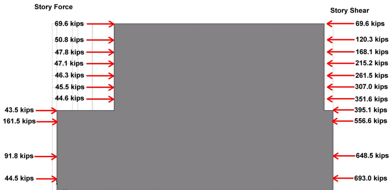
Figure 4: Diagram of Wind Forces Acting in the North/South Direction
