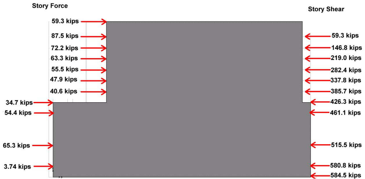
Figure 5: Diagram of Seismic Story Forces and Shears
